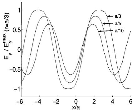
FIG. 8. Electric field at the QCA surface for three different values of wire radius. As the wire radius increases, the amplitude of the field becomes larger since more charge is on each wire at a specific voltage. As the radius decreases, the wave shape becomes more pointed, reflecting the more definite position of each wire underneath the surface.
