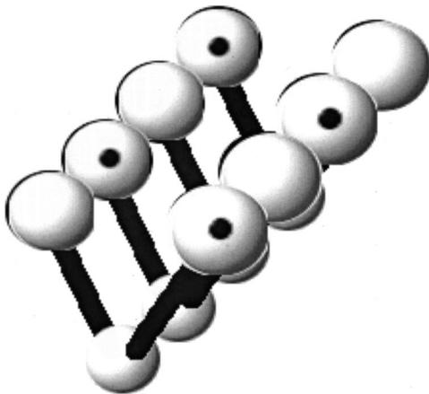
FIG. 2. Schematic of two molecular QCA cells, each with four quantum dots on the top plane used to reflect the polarity of the cell and two dots in the lower plane used to contain the mobile charges when the cell is in a null state. Neighboring cells tend to align their polarities as shown in the figure.
