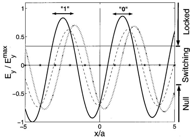
Fig. 5. Value of the clocking field at the QCA surface. Snapshots at different times are depicted by the dotted lines to indicate how the field shifts. Cells on the QCA surface with an applied electric field greater than a critical value will be in a locked state that will be used to store binary information. Over time, the locked state propagates along the  $x$  axis, transporting binary information.
