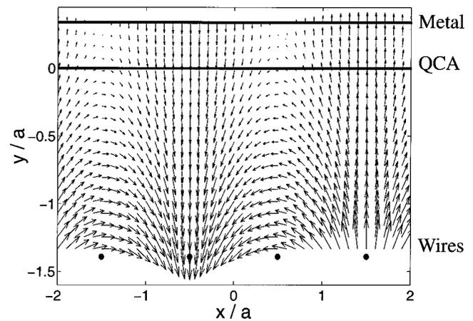
Fig. 6. Electric field distribution between the buried wires and the grounded conductor. The arrows show the direction of the vector field and that the intensity of the field at the QCA surface decreases as it is moved further from the wires.
