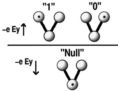
FIG. 1. Cross section of a QCA half cell showing two different states it can exist in. The state is determined by a  $\hat{y}$  directed electric field that either pushes the electrons into a locked state, sucks them down into the null state, or switches them in between. The locked state has two degenerate polarities shown here to represent a binary 1 or 0.
