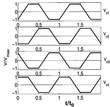
FIG. 4. Four-phase clocking signal applied to four adjacent buried wires. Each wire has a voltage that raises and lowers linearly in order to adiabatically switch the QCA cells above it, that is, switch the cells while keeping them in their ground state. Adjacent wires have a  $\pi/2$  phase shift so that every fourth wire has an identical signal. This method will induce a roughly sinusoidal clocking field that propagates along the QCA surface.
