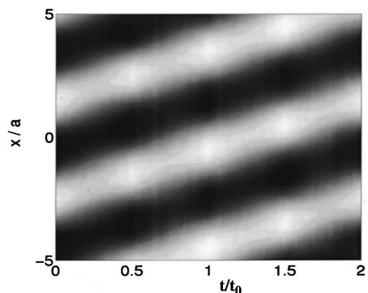
Fig. 7. Electric field at the QCA surface as a function of both time and position. A vertical cross section will show the field at a given time and will be oscillatory as shown in Fig. 5. The bright bands correspond to cells that will be driven into locked states. A continuity of these bands over time ensures that locked states and therefore data will proceed across the surface without interruption.
